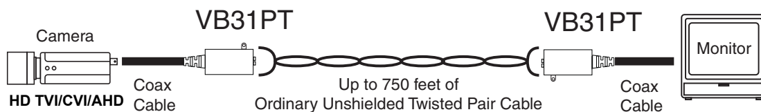
Basic Twisted Pair Video Transmission System
